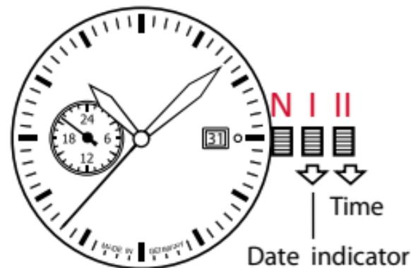
**Date adjustment:** Pull out the crown till position 1 and adjust the date by turning it counter-clockwise, then push the crown back into its neutral position [N].
