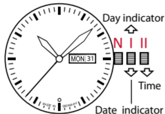
**Time adjustment:** Pull out the crown at position 2 and adjust the time by turning it counter-clockwise, then push the crown back into its neutral position [N].
